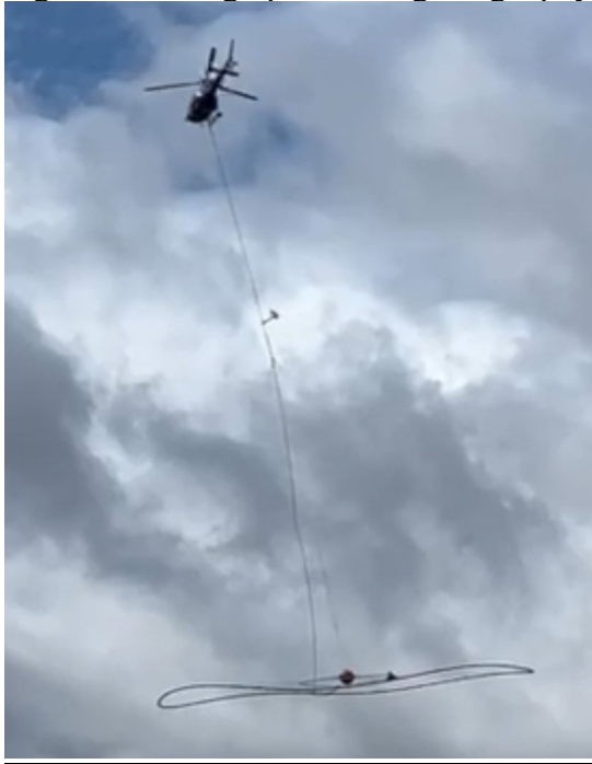
Figure 2: Photograph showing the geophysics array slung under a helicopter.
